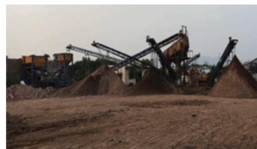
The processing plant's conveyor and crusher setup
