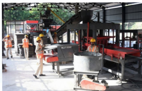
Recycled-aggregate processing and paver-block production line
