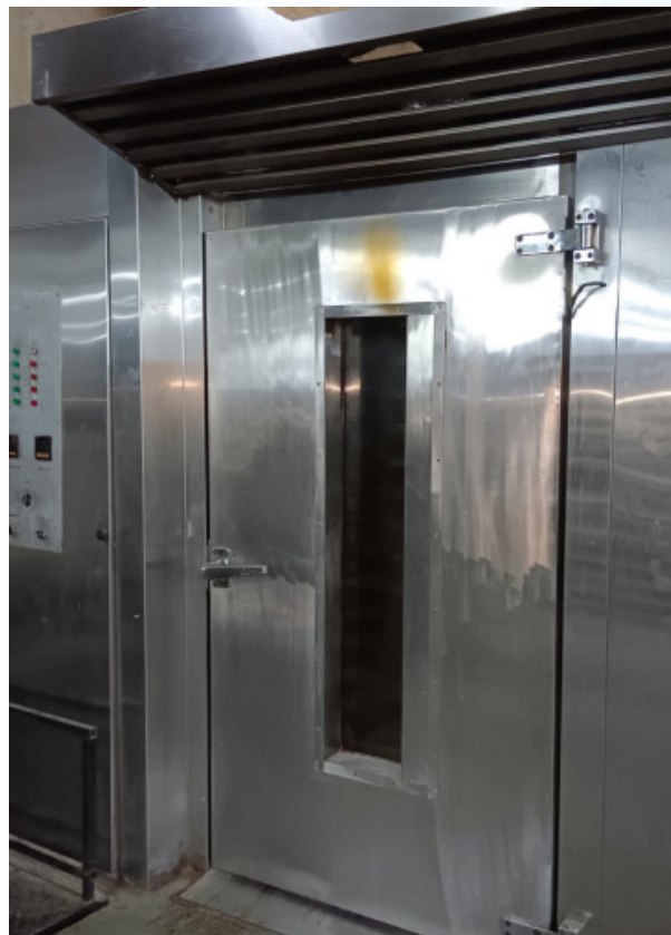
After — a clean-fuel (PNG / electric) rotary bakery oven
