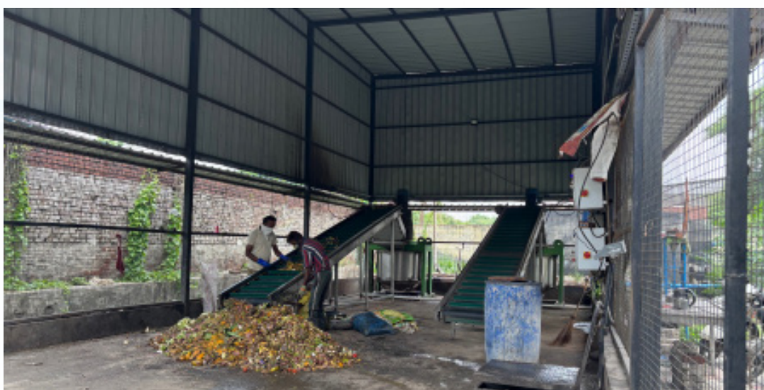
Segregated wet waste fed to the processing line at the Bio-Methanation Plant, Gobindgarh
