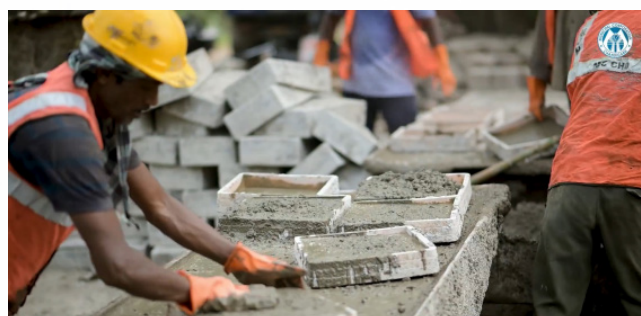
Manufacture of paver blocks from recycled C&D material
