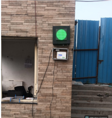
On-site sensor with LED indicator showing green (within threshold) and the monitoring unit below
